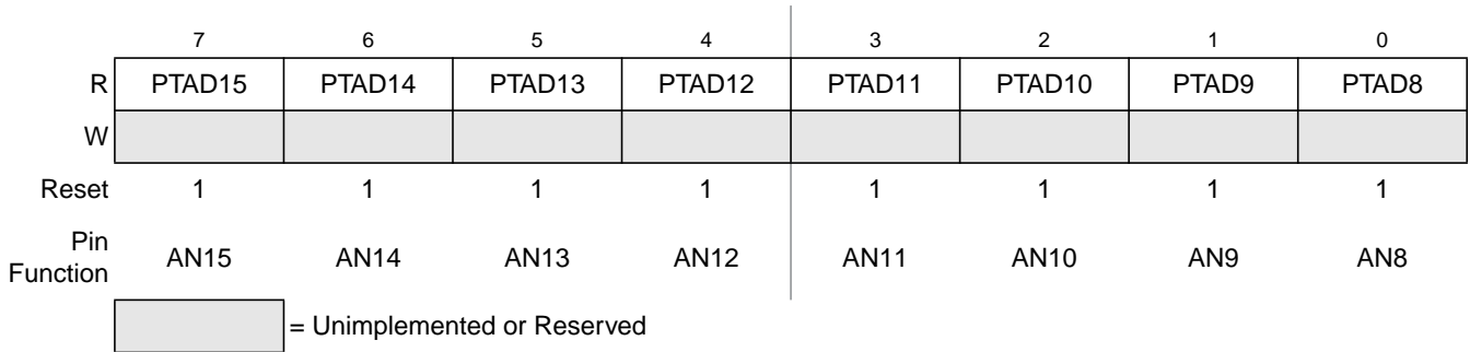
Figure 4-16. Port Data Register 0 (PORTAD0)
