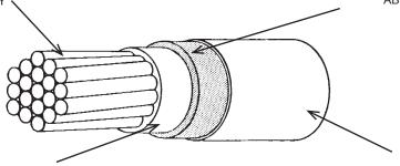
PRIMARY INSULATION - RADIATION-CROSSLINKED, MODIFIED PVDF COLOR - NATURAL PRIMARY JACKET - RADIATION-CROSSLINKED, MODIFIED ETFE
