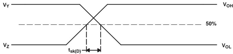
**Figure 5. Definition of Intra-Pair Differential Skew**
