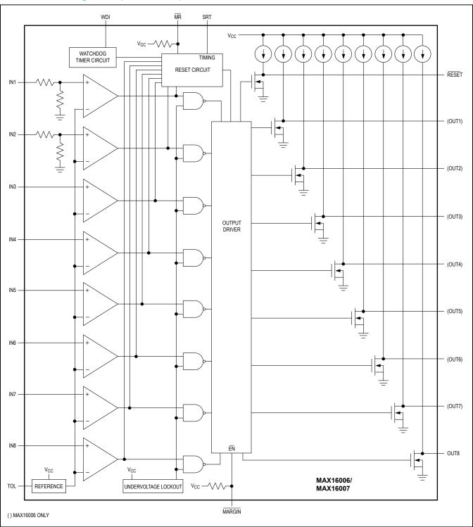
Figure 5. MAX16006C/MAX16007C Functional Diagram
