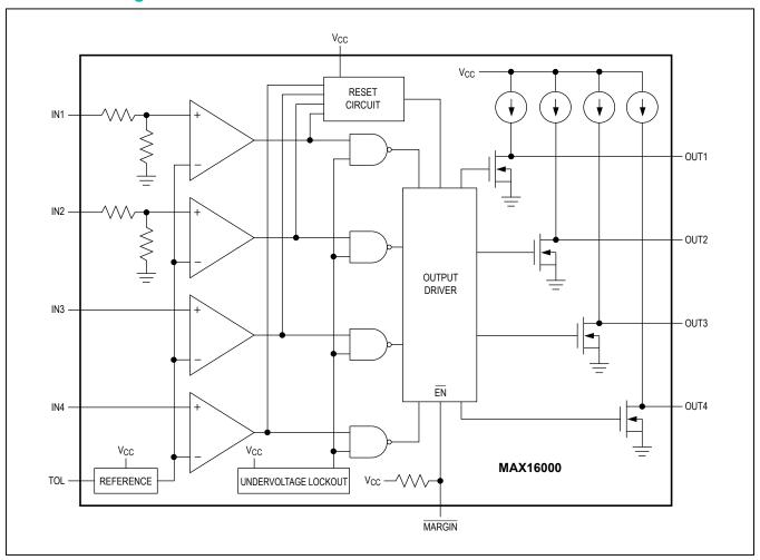
Figure 1. MAX16000D Functional Diagram
