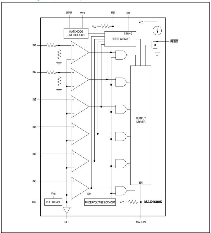
Figure 4. MAX16005C Functional Diagram
