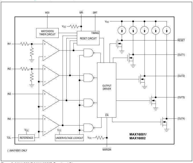
Figure 2. MAX16001D/MAX16002D Functional Diagram
