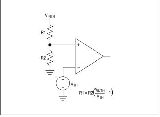
Figure 10. Setting the Adjustable Input
