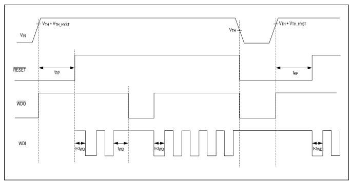
Figure 13.  $\overline{WDO}$  Timing Related to  $V_{TH}$  and  $t_{RP}$
