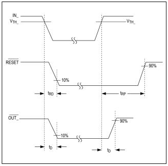
Figure 12. Output Timing Diagram
