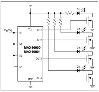
Figure 7. V<sub>CC</sub> Bar-Graph Monitoring
