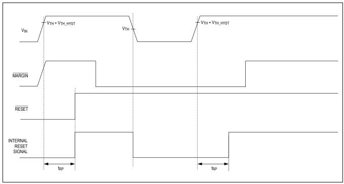
Figure 15. Margin Output Disable (MARGIN) Affect on RESET Outside tree
