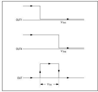
Figure 9. Output Response of Window Detector Circuit
