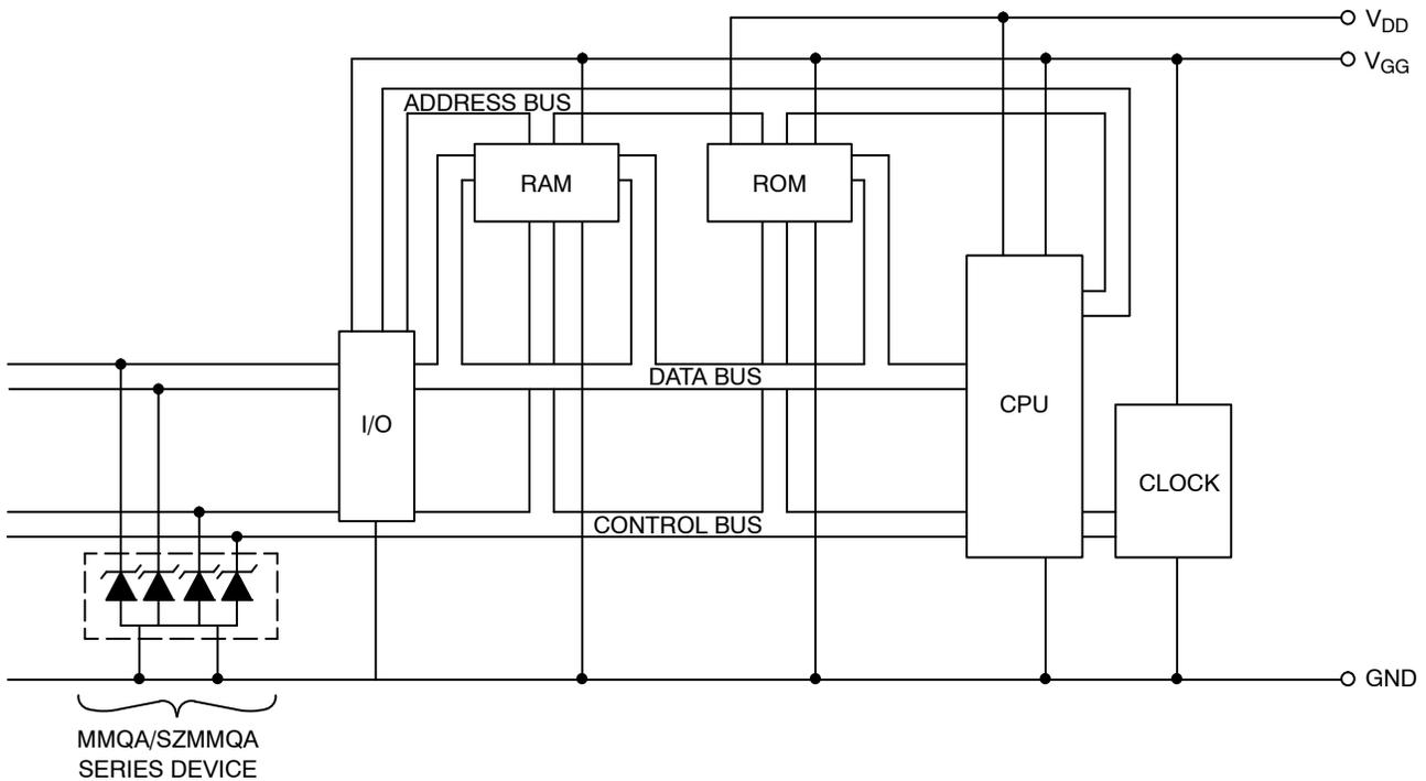
Figure 10. Microprocessor Protection
