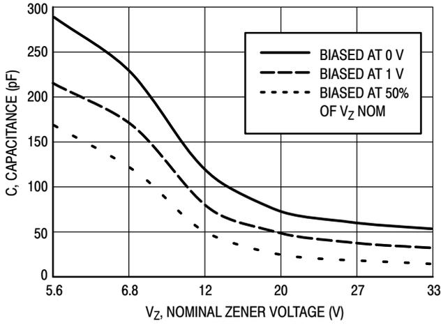
Figure 1. Typical Capacitance
