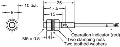
\*2.9-dia. vinyl-insulated round cable with 3 conductors (Conductor cross section: 0.14 mm<sup>2</sup>, Insulator diameter: 2.9 mm), Standard length: 2 m
