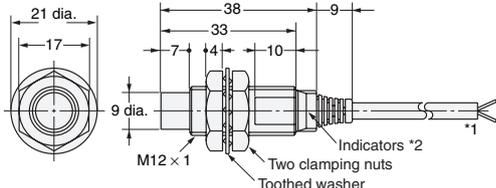
\*1. 4-dia. vinyl-insulated round cable with 2 conductors (Conductor cross section: 0.3 mm<sup>2</sup>, Insulator diameter: 1.3 mm), Standard length: 2 m
