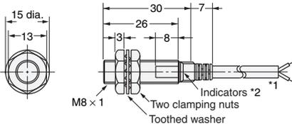
\*1. 4-dia. vinyl-insulated round cable with 2 conductors (Conductor cross section: 0.3 mm<sup>2</sup>, Insulator diameter: 1.3 mm), Standard length: 2 m
