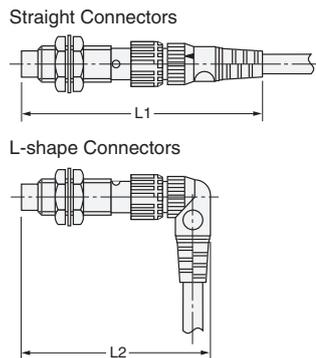
**Dimensions with the XS2F Connected (Unit: mm)**
