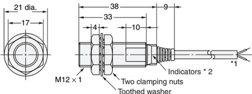
\*1. 4-dia. vinyl-insulated round cable with 2 conductors (Conductor cross section: 0.3 mm<sup>2</sup>, Insulator diameter: 1.3 mm), Standard length: 2 m
