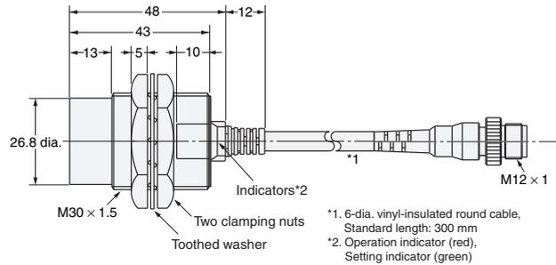
**Dimensions for Proximity Sensors with Sensor I/O Connectors**
