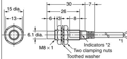
\*1. 4-dia. vinyl-insulated round cable with 2 conductors (Conductor cross section: 0.3 mm<sup>2</sup>, Insulator diameter: 1.3 mm), Standard length: 2 m
