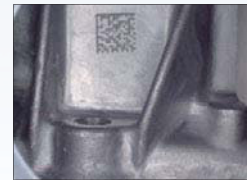
Stable Detection for Metal Surfaces Subject to Gloss and Inconsistent Lighting
