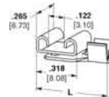
E — Reversible Flag for Hermetic Tabs, Side Feed
