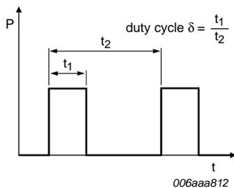
Fig 17. Duty cycle definition
