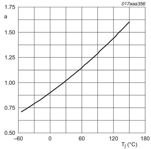
$$a = \frac{R_{DS(on)}}{R_{DS(on)(25\text{ °C})}}$$
