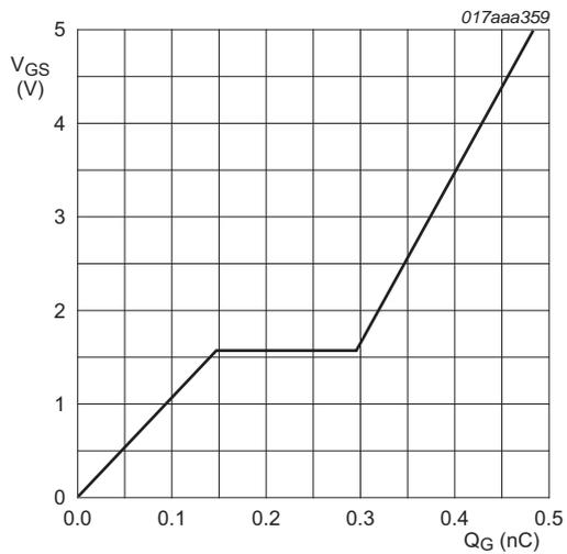
$I_D = 0.5 \text{ A}; V_{DS} = 10 \text{ V}; T_{amb} = 25 \text{ }^\circ\text{C}$
