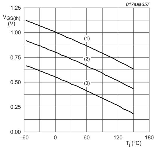
$I_D = 0.25\text{ mA}; V_{DS} = V_{GS}$
