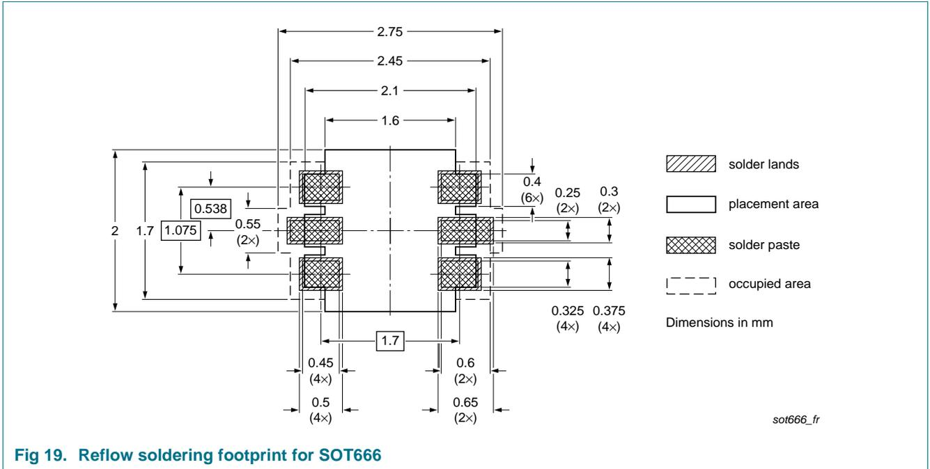
**Fig 19. Reflow soldering footprint for SOT666**
