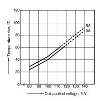
2-(4). Coil temperature rise (2 Form C/DC type) Measured portion: Inside the coil
