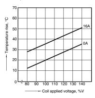
2-(3). Coil temperature rise (2 Form C/AC type) Measured portion: Inside the coil
