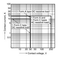
1-(2). Max. switching capacity (2 Form C)
