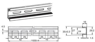
A total of twelve 25 × 4.5 elliptic holes is provided with six holes cut from each track end at a pitch of 10 mm.
