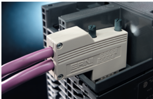
Integral T function, bus in, bus out
