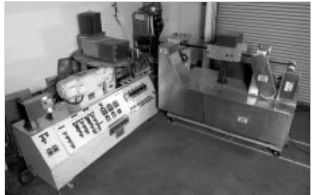
▲ Thermoplastic extruder for microwave absorbing thermoplastic products.
