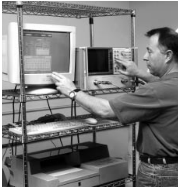
▲ Computer controlled network analyzer provides amplitude and phase measurements on microwave absorbers.
