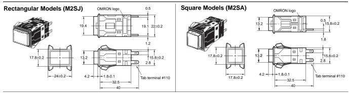
$\textbf{Note:} \ \ \textbf{Unless otherwise specified, a tolerance of } \pm 0.4 \ \text{mm applies to all dimensions.} \ \ \textbf{Recommended panel thickness: 1 to 4 mm}$
