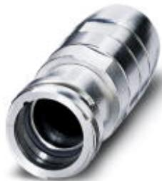
Sleeve housing for coupler connector, straight, Bayonet locking, M23, shielded: yes, cable diameter range: 2 mm ... 14.5 mm
