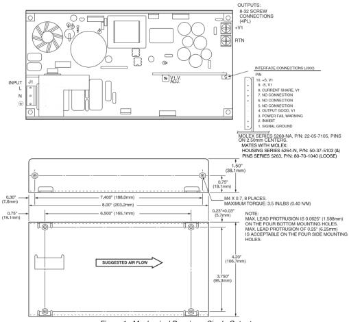
Figure 1. Mechanical Drawing - Single Output
