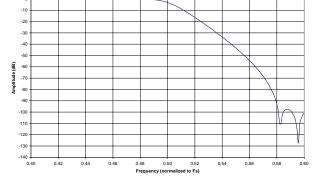
Figure 2. Single Speed Mode Transition Band
