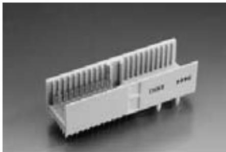
The ERmet male connector type M provides a maximum of 77 contacts in 7 rows by 11 positions. The two outer rows, z and f are for the shielding contacts of the male connector, along with 3 contact positions for special power or coax contacts. This type contains a multifunction cavity for coding and pre-alignment in the center position. This connector is designed to be used alone or in conjunction with either a type B, C, L, or N ERmet connector.
