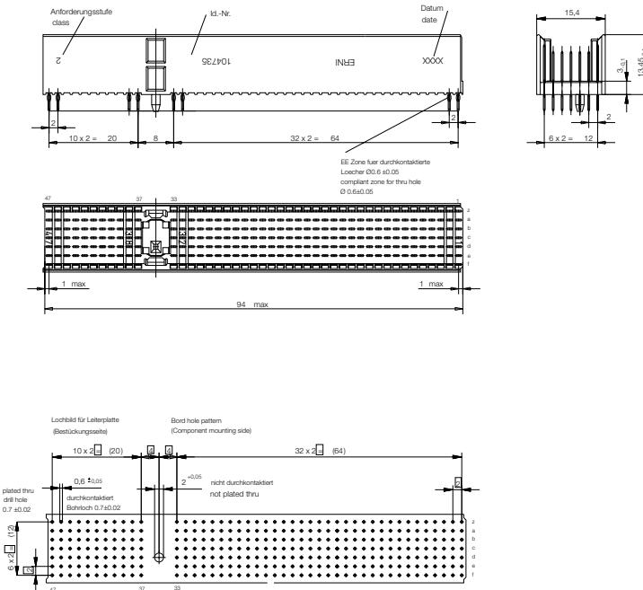
Note: The numbering on the connectors themselves is in accordance with the IEC 61076-4-101 standard. All dimensions in mm.
