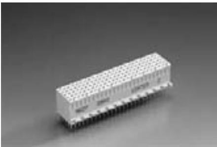
The ERmet type B vertical female connector provides 125 contacts in a 5 row x 25 position fully loaded configuration. Versions with optional "z" and "f" row shields are available as well as extended terminals for use in stacking applications with rear shrouds.
