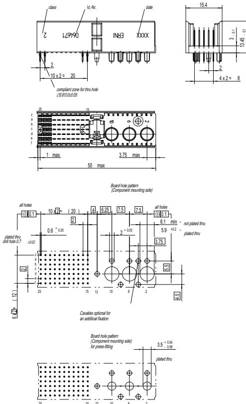
Note: The numbering on the connectors themselves is in accordance with the IEC 61076-4-101 standard. All dimensions in mm.
