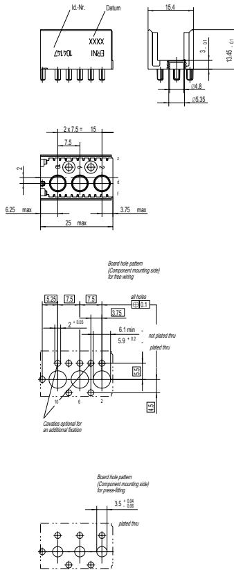
Note: The numbering on the connectors themselves is in accordance with the IEC 61076-4-101 standard. All dimensions in mm.
