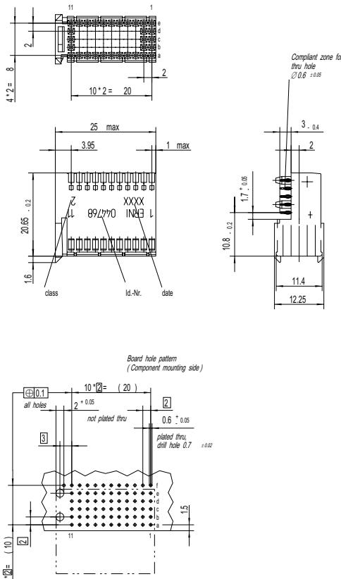
Note: The numbering on the connectors themselves is in accordance with the IEC 61076-4-101 standard. All dimensions in mm.
