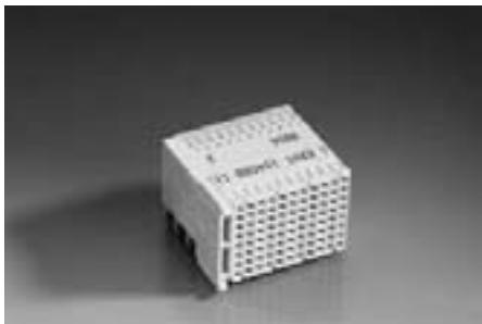
The ERmet type F female connector provides 88 signal contacts and 22 ground shield contacts in an 8 row x 11 position fully loaded configuration.
