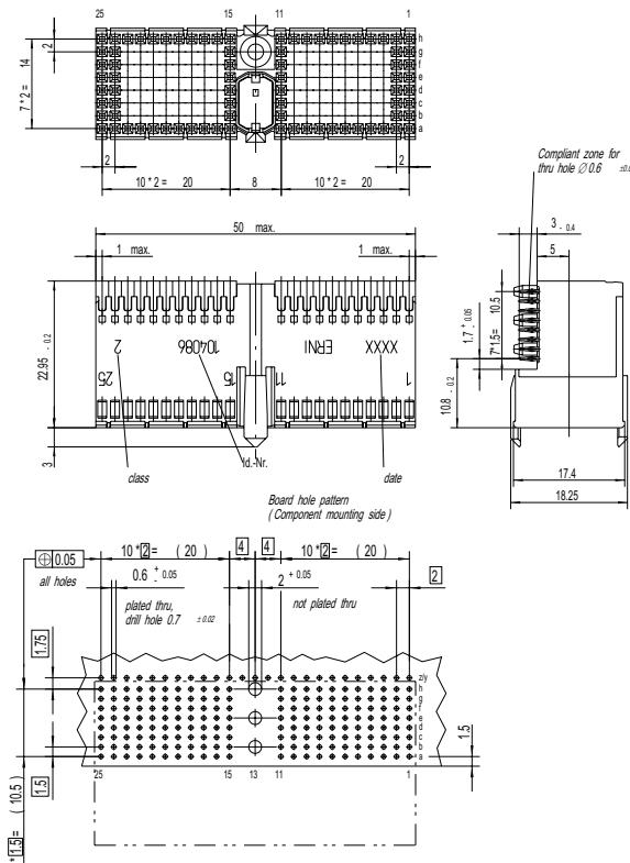
Note: The numbering on the connectors themselves is in accordance with the EC 61076-4-101 standard. All dimensions in mm.
