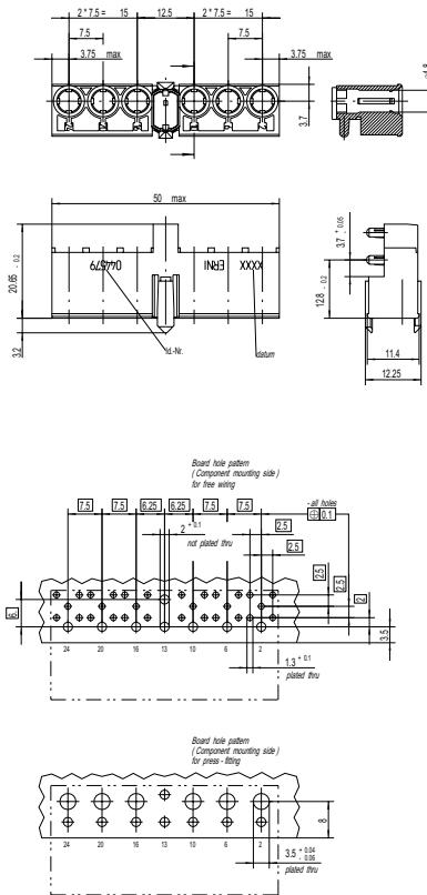
Note: The numbering on the connectors themselves is in accordance with the IEC 61076-4-101 standard. All dimensions in mm.
