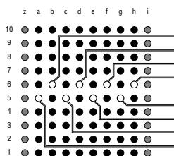
● ground   ○ signal pin   ○ shielding pin
