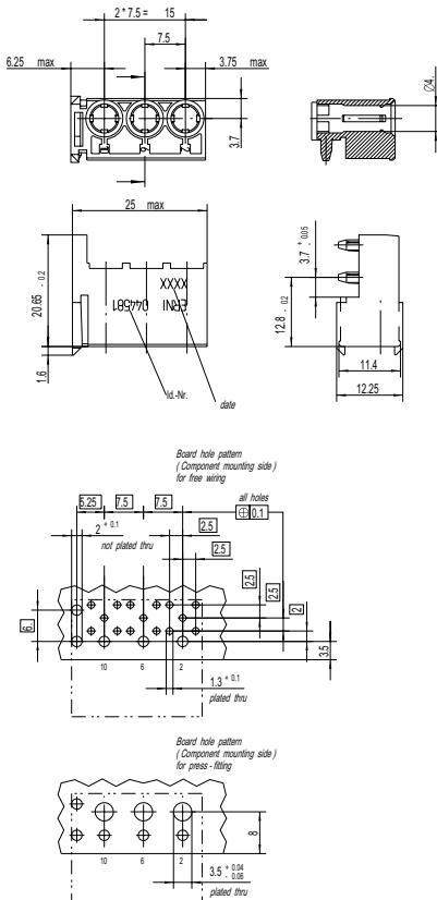
Note: The numbering on the connectors themselves is in accordance with the IEC 61187-6-4-101 standard. All dimensions in mm.
