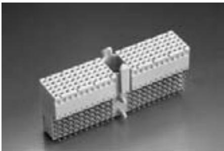
The ERmet type A female connector provides 110 contacts in a 5 row x 25 position (3 positions used by multifunction cavity), fully loaded configuration. This connector is used in the J1 and J4 positions of the CompactPCI® daughter card. The connector is designed for gas tight, pressfit installation and is provided in two different configurations: with integrated upper ground return shields and without integrated upper ground return shields. Lower ground return shields are available separately.
