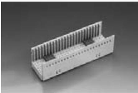
The ERmet™ shroud type B is possible for a maximum of 175 contacts in 7 rows by 25 positions. The two outer rows, z and f are for the shielding contacts of the female connector. For this type, without multifunction block for coding and pre-alignment, we recommend use only in combination with types A or C.
