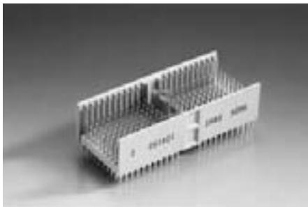
The ERmet type D vertical male connector provides up to 176 signal contacts and 44 ground shield contacts in 8+2 row x 25 position (3 positions used by multifunction cavity), fully loaded configuration. With 15 different standard pin lengths to choose from, this is one of the most versatile connectors available. The connector is designed for gas tight pressfit installation.
