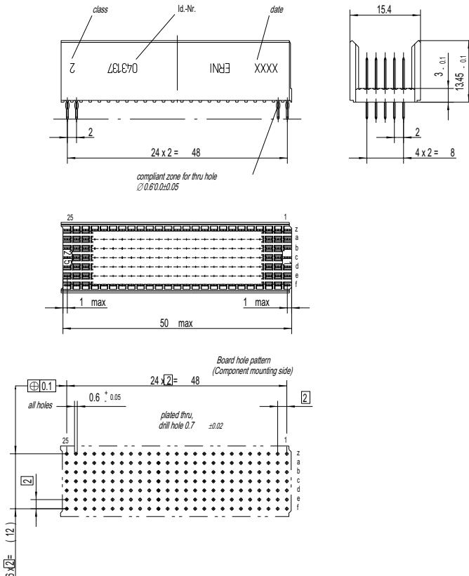
Note: The numbering on the connectors themselves is in accordance with the IEC 61076-4-101 standard. All dimensions in mm.
