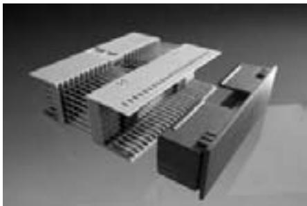
The dust and protection cover for the male connectors for the ERmet™ 2.0 mm connector system acc. to IEC 61076-4-101 protect the mating area at the frontside of the backplane and what is more important the transfer area on the rear side of the backplane against damage of the contacts. They are also a protection for transportation and against dust. The dust and protection cover is available in two versions for type A, B, AB and for type D, E, DE with or without grip.
