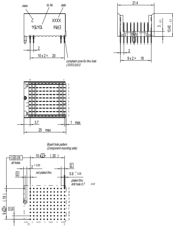
**Note:** The numbering on the connectors themselves is in accordance with the IEC 61076-4-101 standard. All dimensions in mm
