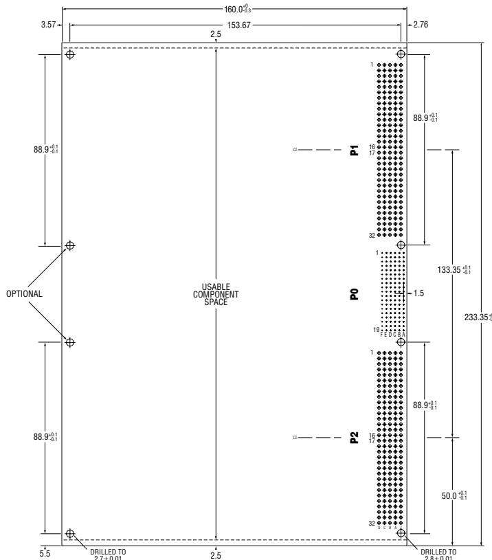
Note that the numbering of the P0 connector conforms to IEEE 1101.1 and 1101.10 and is from the top down. This also is the same numbering scheme established by the connector standard IEC 61076-4-101.
