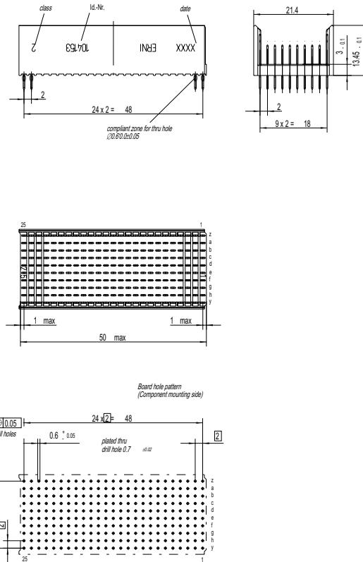
Note: The numbering on the connectors themselves is in accordance with the IEC 61076-4-101 standard. All dimensions in mm.
