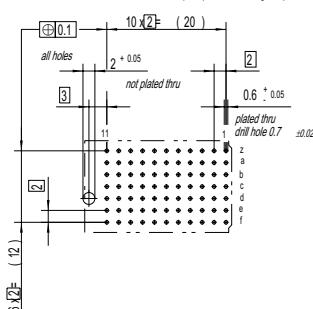
Note: The numbering on the connectors themselves is in accordance with the IEC 61076-4-101 standard. All dimensions in mm.
