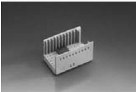
The ERmet shroud type C is possible for a maximum of 77 contacts in 7 rows by 11 positions with the length of 25 mm. The two outer rows, z and f are for the shielding contacts of the female connector.
