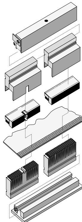
Modular press-fit tool for female connector modules 5+2
