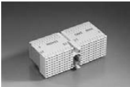
The ERmet type D female connector provides 176 signal contacts and 44 ground shield contacts in a 8 row x 25 position (3 positions used by multifunction cavity), fully loaded configuration.
