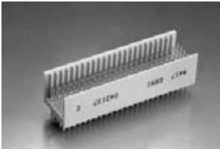
The ERmet CompactPCI type B vertical male connector provides 125 signal contacts and 50 ground shield contacts in a 5+2 row x 25, fully loaded configuration. With 15 different standard pin lengths to choose from, this is one of the most versatile connectors available. The connector is designed for gas tight pressfit installation.
