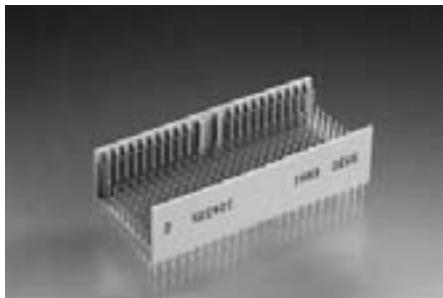
The ERmet type DE vertical male connector provides 200 signal contacts and 44 ground shield contacts in a 8+2 row x 25 position fully loaded configuration. With 15 different standard pin lengths to choose from, this is one of the most versatile connectors available. The connector is designed for gas tight pressfit installation.
