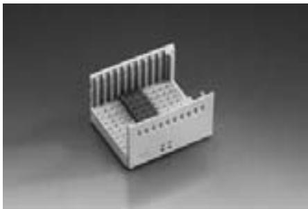
The ERmet shroud type F is possible for a maximum of 110 contacts in 10 rows by 11 positions with the length of 25 mm. The two outer rows, z and y are for the shielding contacts of the female connector.
