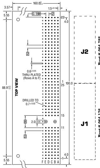
*Note that the backplane and daughter card are numbered in accordance with the CompactPCI® specification. The numbering on the connectors themselves is different and in accordance with the IEC 61076-4-101 standard.*
