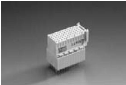
The ERmet type C vertical female connector provides 55 contacts in a 5 row x 11 position fully loaded configuration. Versions with optional "z" and "f" row shields are available as well as extended terminals for use in stacking applications with rear shrouds.
