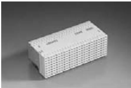
The ERmet type E female connector provides 200 signal contacts and 50 ground shield contacts in a 8 row x 25 position fully loaded configuration.
