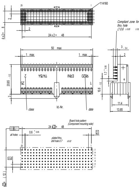
Note: The numbering on the connectors themselves is in accordance with the IEC 61076-4-101 standard. All dimensions in mm.
