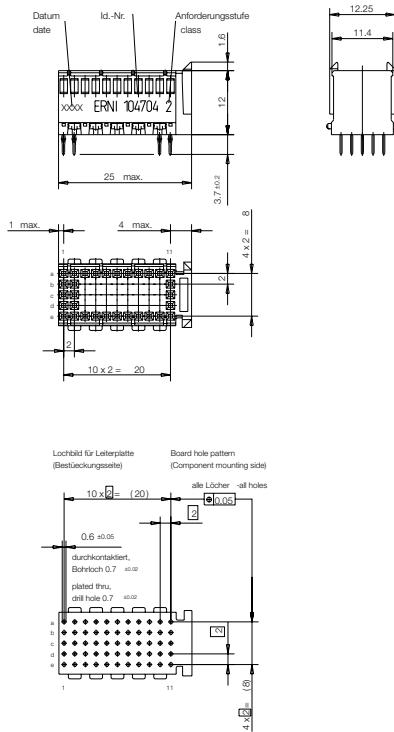
Note: The numbering on the connectors themselves is in accordance with the IEC 61076-4-101 standard. All dimensions in mm.
