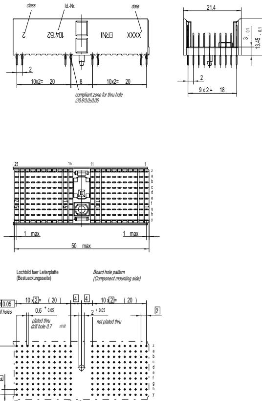
Note: The numbering on the connectors themselves is in accordance with the IEC 61076-4-101 standard. All dimensions in mm.
