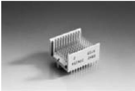
The ERmet type F vertical male connector provides 88 signal contacts and 22 ground shield contacts in a 8+2 row x 11, fully loaded configuration. With 15 different standard pin lengths to choose from, this is one of the most versatile connectors available. The connector is designed for gas tight pressfit installation.
