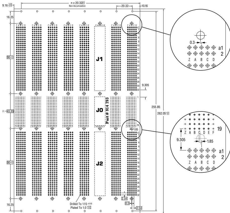
Note that the numbering of the P0 connector conforms to IEEE 1101.1 and 1101.10 and is from the top down. This also is the same numbering scheme established by the connector standard IEC 61076-4-101.
