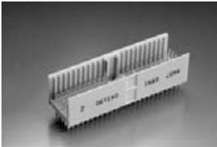
The ERmet type A vertical male connector provides 110 signal contacts and 44 ground shield contacts in 5+2 row x 25 position (3 positions used by multifunction cavity), fully loaded configuration. This connector is used in the P1 and P4 positions of a CompactPCI® backplane. With 15 different standard pin lengths to choose from, this is one of the most versatile connectors available. The connector is designed for gas tight pressfit installation.
