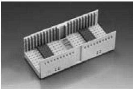
The ERmet shroud type D is possible for a maximum of 220 contacts in 10 rows by 25 positions with the length of 50 mm. The two outer rows, z and y are for the shielding contacts of the female connector. This type contains a multi-function block for coding and pre-alignment which uses 3 positions
