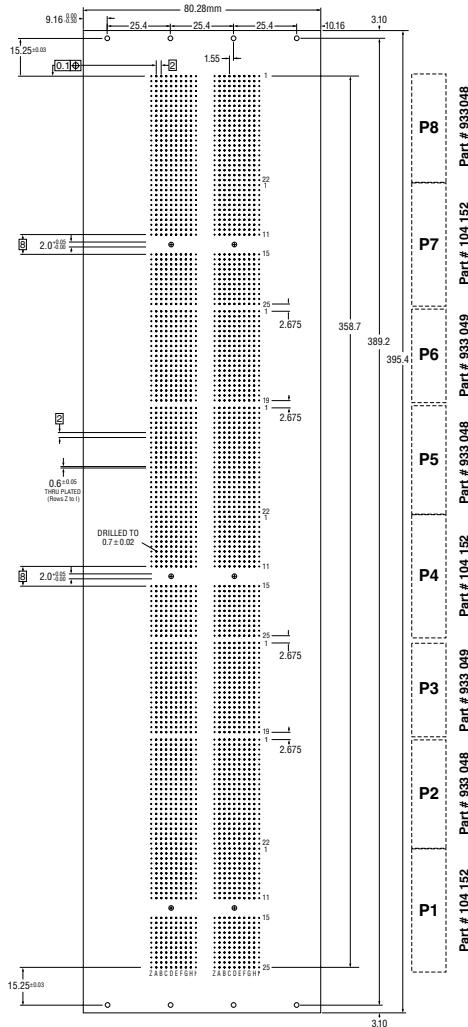
Note that the numbering scheme conforms with the Type V numbering as defined in VITA30-199x Draft 0.5 dated 9 June 1999 and is from the top down. This numbering scheme is identical to the numbering established for the connector within the IEC 61076-4-101 standard.
