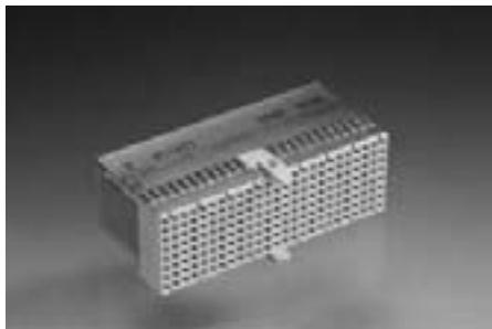
The ERmet type DE female connector provides 200 signal contacts and 25 ground shield contacts in an 8 row x 25 position fully loaded configuration.
