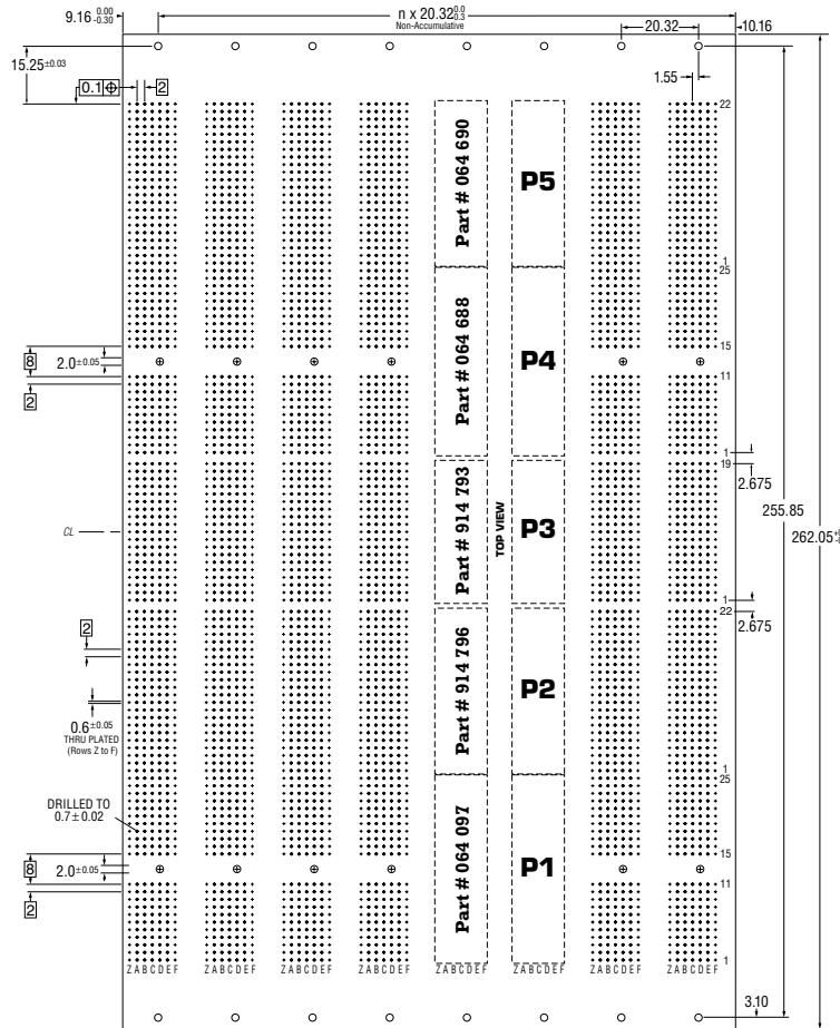
Note that the backplane is numbered in accordance with the CompactPCI® specification. The numbering on the connectors themselves is different and in accordance with the IEC 61076-4-101 standard.
