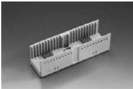
The ERmet shroud type A is possible for a maximum of 175 contacts in 7 rows by 25 positions. The two outer rows, z and f are for the shielding contacts of the female connector. This type contains a multifunction block for coding and pre-alignment which uses 3 positions. For CompactPCI applications the shroud type A is used on the position rP1 and rP4.
