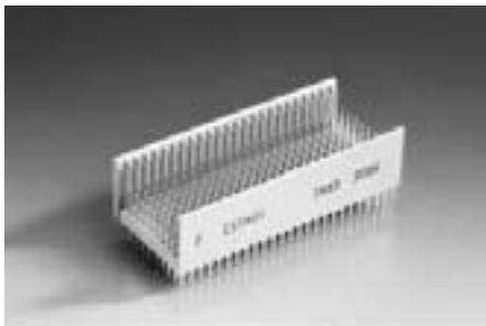
The ERmet type E vertical male connector provides 200 signal contacts and 50 ground shield contacts in an 8+2 row x 25 position fully loaded configuration. This connector is also available in an 8+2 row x 22 positions and 8+2 row x 19 positions. With 15 different standard pin lengths to choose from, this is one of the most versatile connectors available. The connector is designed for gas tight pressfit installation.
