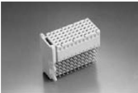
The ERmet type C female connector provides 55 contacts in a 5 row x 11 position fully loaded configuration. The connector is designed for gas tight, pressfit installation and is provided in two different configurations: with integrated upper ground return shields and without integrated upper ground return shields. Lower ground return shields are available separately.
