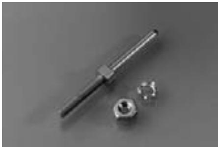
The optional applicable guide pin for the 10 row ERmet type D connector made of stainless steel is suited for the secure pre-centering when mating. The guide pin will be screwed with the connector and the pcb after the male connector has been pressed-in.
