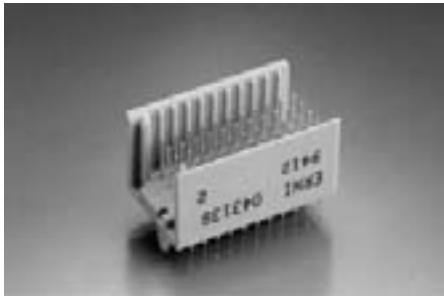
The ERmet type C vertical male connector provides 55 signal contacts and 22 ground shield contacts in 5+2 row x 11 position, fully loaded configuration. With 15 different standard pin lengths to choose from, this is one of the most versatile connectors available. The connector is designed for gas tight pressfit installation.
