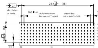
Note: The numbering on the connectors themselves is in accordance with the IEC 61076-4-101 standard. All dimensions in mm.
