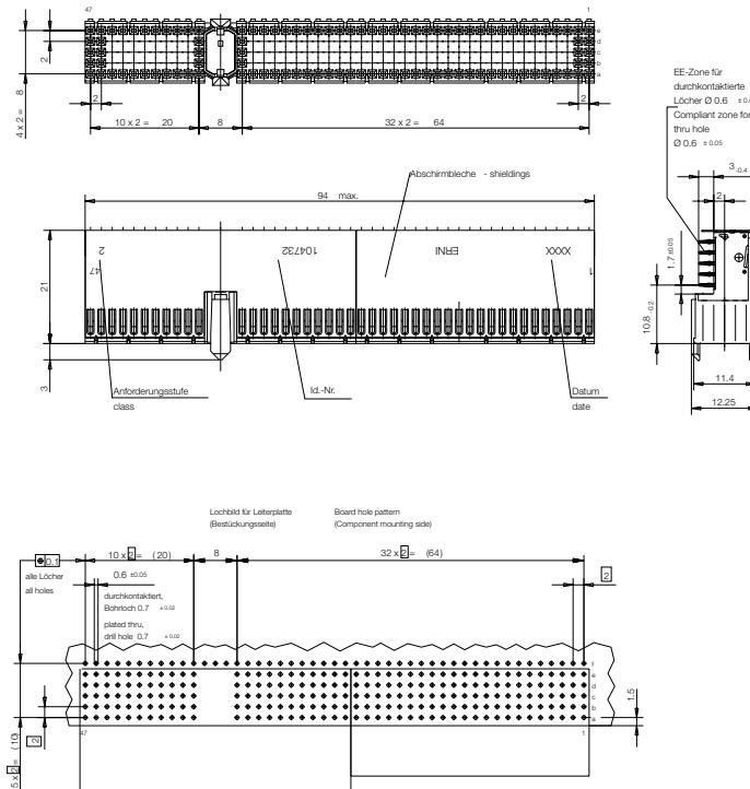
**Note:** The numbering on the connectors themselves is in accordance with the IEC 61076-4-101 standard. All dimensions in mm.
