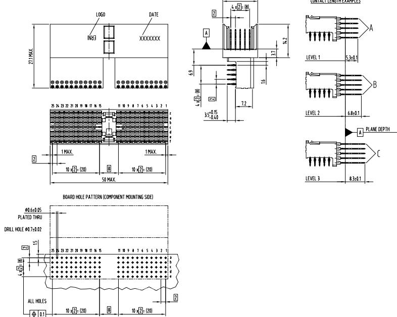
The ERmet type A right angle male connector provides 110 contacts in a 5 row x 25 position (3 positions used by multi-function cavity), fully loaded configuration.
