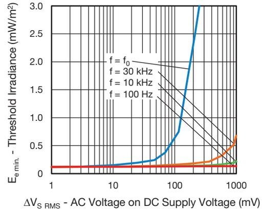
Fig. 7 - Sensitivity vs. Supply Voltage Disturbances
