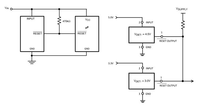
Figure 9. Microprocessor Reset Circuit
