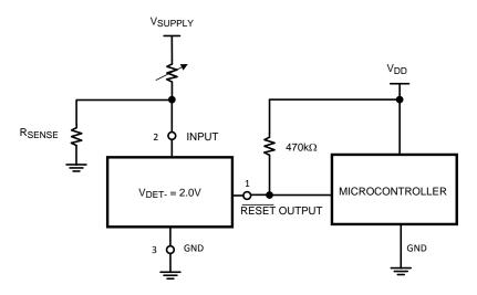
THIS CIRCUIT MONITORS THE CURRENT AT THE LOAD. AS CURRENT FLOW THROUGH THE LOAD, A VOLTAGE DROP WITH RESPECT TO GROUND APPEARS ACROSS R<sub>SENSE</sub> WHERE V<sub>SENSE</sub> = I<sub>LOAD</sub> \* R<sub>SENSE</sub>. THE FOLLOWING CONDITIONS APPLY:
