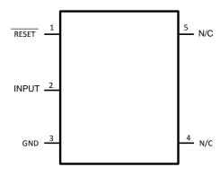
Figure 1. 5-Pin SOT-23 **Top View**
