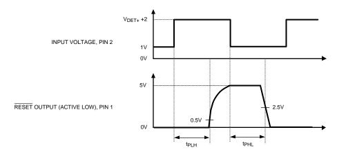
Figure 7. Propagation Delay Timing Diagrams
