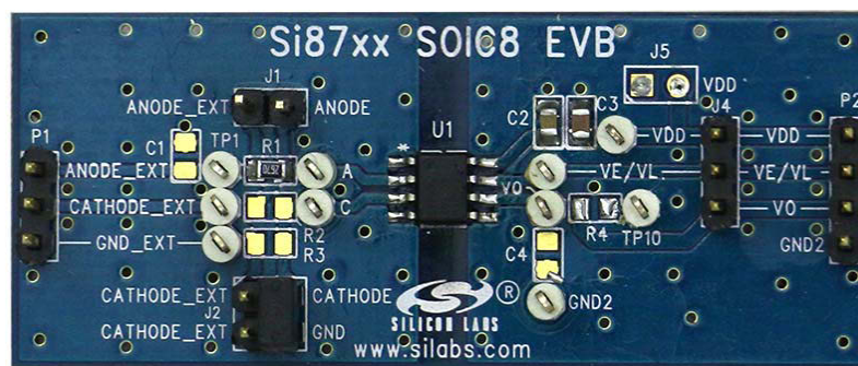
Figure 2. Si871x SOIC8 Evaluation Board Overview
