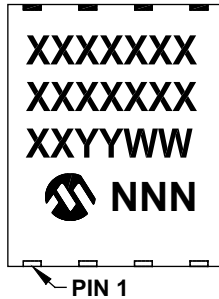
8-Lead PDFN (5x6x1.0 mm)
