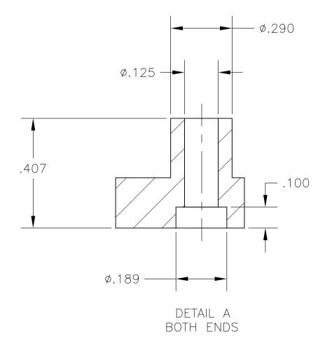
THIS DRAWING IS A CON DIMENSIONS: INCHES  $\bigcirc \sub$ MATERIAL
