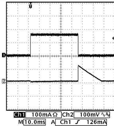
$V_{IN} = 3.6\text{ V}$        $V_{OUT} = 2.6\text{ V}$       0 to 150-mA Load
