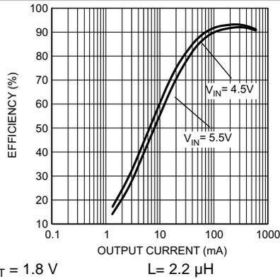
**Figure 18. Efficiency vs Output Current (Forced PWM Mode)**
