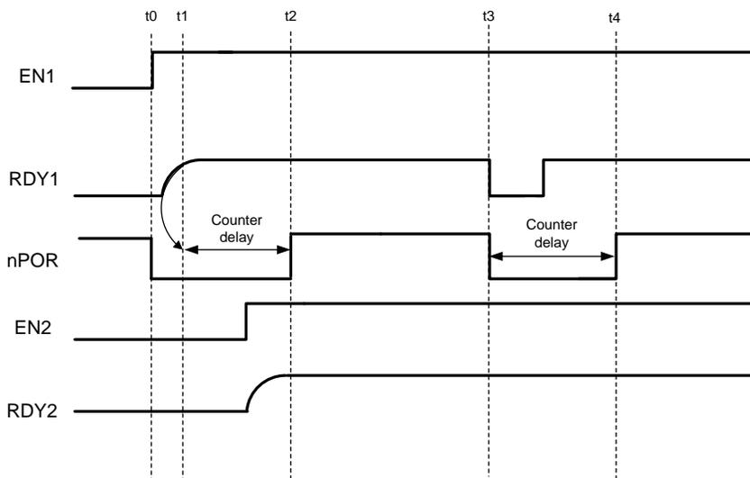
Figure 36. Faults Occurring in Counter Delay After Start-Up
