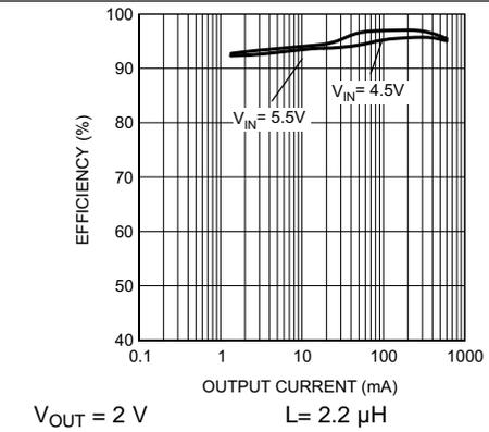
**Figure 21. Efficiency vs Output Current (PWM-to-PFM Mode)**
