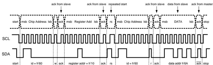
Figure 43. I<sup>2</sup>C Read Cycle
