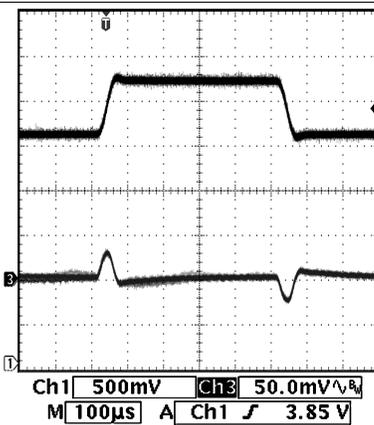
$V_{IN} = 3.6\text{ to }4.2\text{ V}$        $V_{OUT} = 2.6\text{ V}$       300-mA Load
