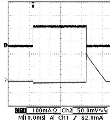
$V_{IN} = 3.6\text{ V}$        $V_{OUT} = 3.3\text{ V}$       0 to 150-mA Load
