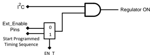
Figure 32. Power Rail Enable Logic
