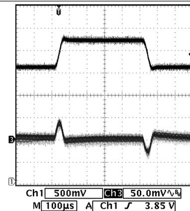
$V_{IN} = 3.6\text{ to }4.2\text{ V}$        $V_{OUT} = 3.3\text{ V}$       300-mA Load
