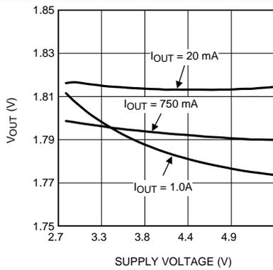
$V_{OUT} = 1.8\text{ V}$
