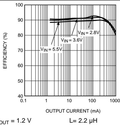
Figure 16. Efficiency vs Output Current (PWM-to-PFM Mode)
