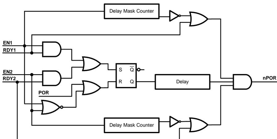
**Figure 38. Design Implementation of the Flexible Power-On Reset**
