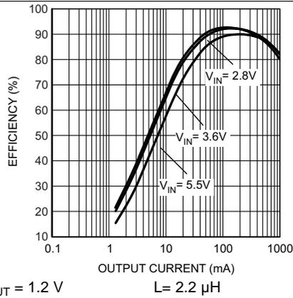
Figure 14. Efficiency vs Output Current (Forced PWM Mode)
