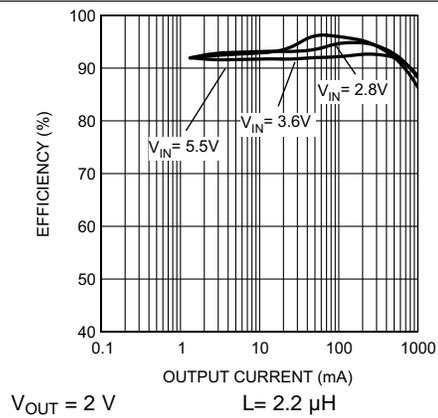
Figure 17. Efficiency vs Output Current (PWM-to-PFM Mode)
