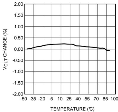
$V_{IN} = 3.6\text{ V}$        $V_{OUT} = 2.6\text{ V}$       100-mA Load
