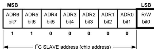
Figure 41. I<sup>2</sup>C Chip Address (see note above)
