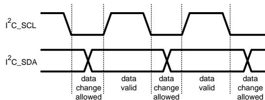
**Figure 39. I<sup>2</sup>C Signals: Data Validity**
