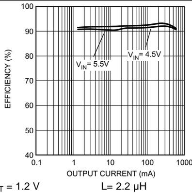
**Figure 20. Efficiency vs Output Current (PWM-to-PFM Mode)**
