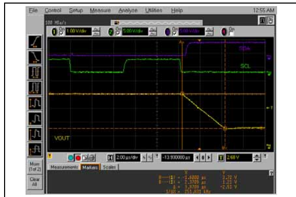
FIGURE 2-99: Half-Scale Settling Time (C00h to 400h) (MCP4726).
