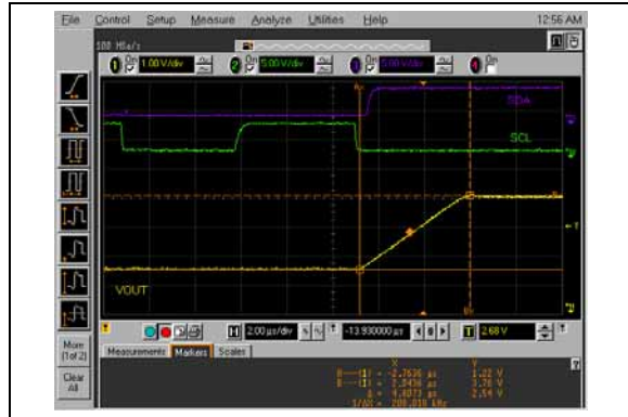
FIGURE 2-98: Half-Scale Settling Time (400h to C00h) (MCP4726).
