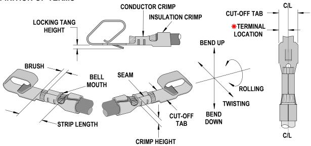
\*Terminal is to be centrally located between the two (2) cut-off edges by 1/2 of the total cut-off tab tolerance.
