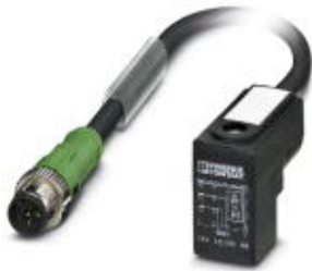
Sensor/actuator cable, 3-position, PUR, black-gray RAL 7021, Plug straight M12, A-coded, on Valve connector C (8 mm), with 1 LED, connected with Z diode, connected with Z diode, cable length: 0.6 m
