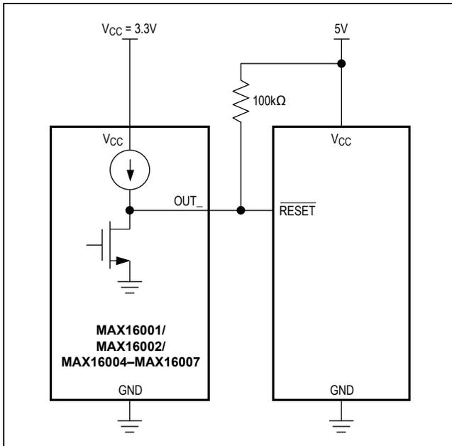
Figure 11. Interfacing to a Different Logic Supply Voltage
