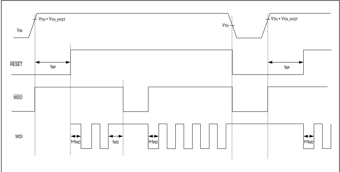
Figure 13.  $\overline{WDO}$  Timing Related to  $V_{TH}$  and  $t_{RP}$
