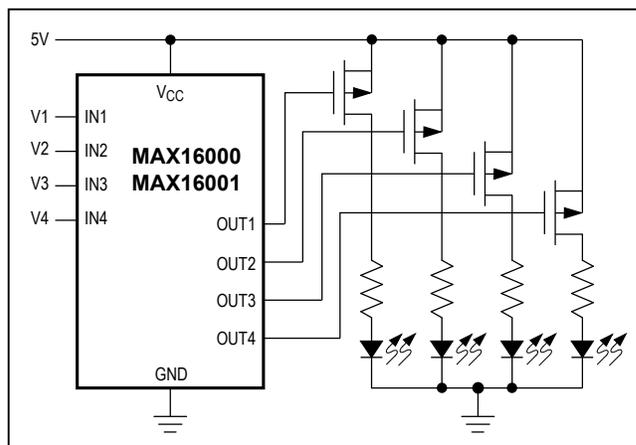
Figure 6. Quad Undervoltage Detector with LED Indicators
