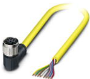
Sensor/actuator cable, 8-position, PVC, yellow, free cable end, on Socket angled M12 SPEEDCON, coding: A, cable length: 5 m
