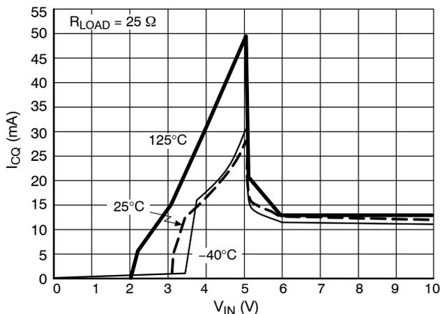
Figure 2. Quiescent Current vs. Input Voltage Over Temperature
