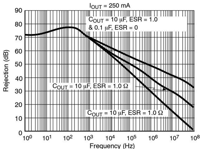
Figure 10. Ripple Rejection
