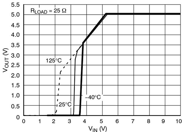
Figure 4. Output Voltage vs. Input Voltage Over Temperature
