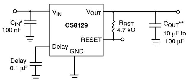
\* $C_{\text{IN}}$  is required if regulator is far from the power source filter.
