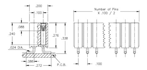
**Description:** Interconnect Socket Surface Mount Socket Accepts .025" - .037" (0,635 - 0,94 mm)dia leads Double Row Surface Mount **Plating Code:**
