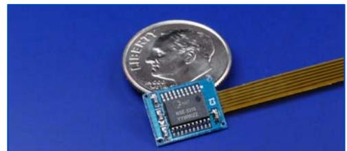
**NSE-5310 position sensor** – closed-loop kits include an NSE-5310 sensor. Evaluate the sensor and/or the performance of a closed-loop SQUIGGLE motor system.
