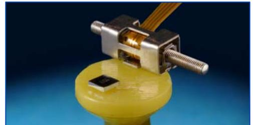
**SQUIGGLE RV motor and driver** – all kits integrate an SQL-RV-1.8 SQUIGGLE RV motor and NSD-2101 drive ASIC into a mechanical and electrical reference design.
