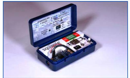
**Developer's kits** demonstrate system performance of an integrated SQUIGGLE motor, NSD-2101 driver and NSE-5310 position sensor.
