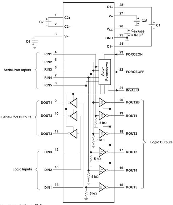
$<sup>^{\</sup>dagger}$  C3 can be connected to  $V_{CC}$  or GND. NOTE A: Resistor values shown are nominal.
