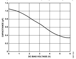
Figure 63. Capacitance vs. Voltage Characteristic
