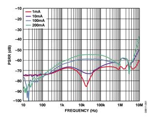
Figure 52. LDO2 PSRR Across Output Load, VIN3 = 5 V, VOUT3 = 3.3 V
