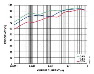
Figure 11. Buck Efficiency vs. Load Current, Across Input Voltage, VOUT1 = 3.3 V, Auto Mode
