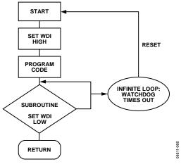
Figure 65. Watchdog Flow Diagram
