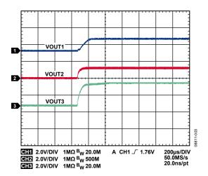
Figure 3. 3-Channel Start-Up Waveforms
