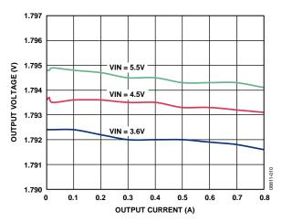
Figure 10. Buck Load Regulation Across Input Voltage, VOUT1 = 1.8 V, PWM Mode
