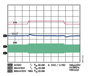
Figure 24. Buck Response to Line Transient, Input Voltage from 4.5 V to 5.0 V, VOUT1 = 3.3 V,  $PWM \, Mode$
