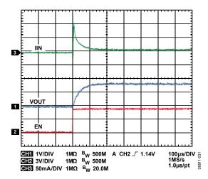
Figure 31. LDO2 Startup, VOUT3 = 3.3 V, IOUT3 = 5 mA
