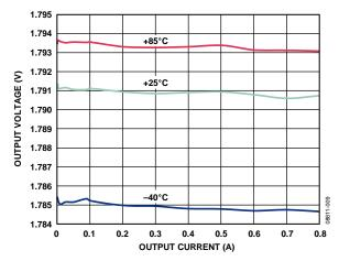
Figure 9. Buck Load Regulation Across Temperature, VOUT1 = 1.8 V, PWM Mode
