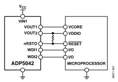
Figure 66. Typical Applications Circuit
