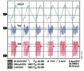
Figure 20. Typical Waveforms, VOUT1 = 3.3 V, I<sub>OUT1</sub> = 30 mA, Auto Mode
