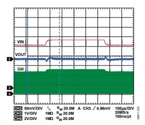
Figure 25. Buck Response to Line Transient,  $V_{\rm IN}$  = 4.5 V to 5.0 V, VOUT1 = 1.8 V, PWM Mode
