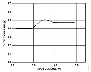
Figure 18. Buck DC Current Capability vs. Input Voltage, VOUT1 = 1.8 V
