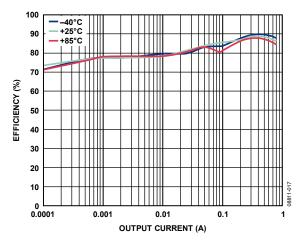
Figure 17. Buck Efficiency vs. Load Current, Across Temperature, VOUT1 = 1.8 V, Auto Mode
