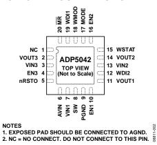
Figure 2. Pin Configuration—View from Top of the Die
