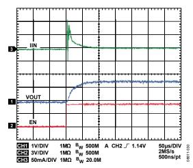
Figure 30. LDO1 Startup, VOUT3 = 1.5 V, IOUT3 = 5 mA
