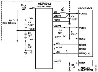
Figure 62. Processor System Power Management with PSM/PWM Control
