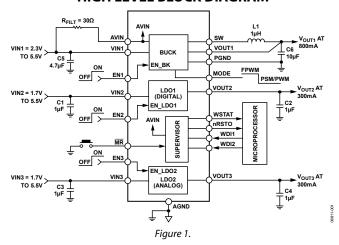
The low quiescent current, low dropout voltage, and wide input voltage range of the ADP5042 LDOs extend the battery life of portable devices. The two LDOs maintain power supply rejection greater than 60 dB for frequencies as high as 10 kHz while operating with a low headroom voltage.
