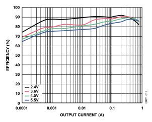
Figure 13. Buck Efficiency vs. Load Current, Across Input Voltage, VOUT1 = 1.8 V, Auto Mode
