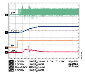
Figure 6. Buck Startup, VOUT1 = 1.8 V,  $I_{OUT2} = 20 \text{ mA}$
