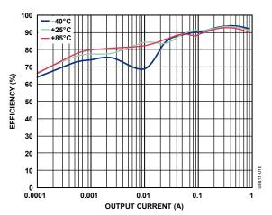
Figure 16. Buck Efficiency vs. Load Current, Across Temperature, VOUT1 = 3.3 V, Auto Mode
