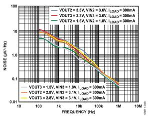
Figure 49. LDO1 vs. LDO2 Noise Spectrum
