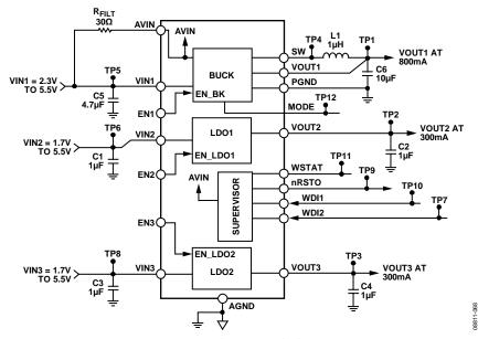
Figure 67. Evaluation Board Schematic
