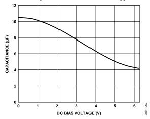
Figure 61. Typical Capacitor Performance
