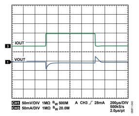
Figure 40. LDO2 Response to Load Transient, IOUT3 from 1 mA to 80 mA, VOUT3 = 3.3 V
