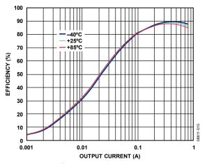
Figure 15. Buck Efficiency vs. Load Current, Across Temperature, VOUT1 = 1.8 V, PWM Mode
