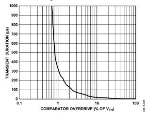
Figure 64. Maximum V<sub>TH</sub> Transient Duration vs. Reset Threshold Overdrive
