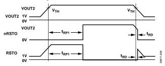
Figure 57. Reset Timing Diagram
