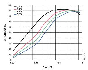
Figure 14. Buck Efficiency vs. Load Current, Across Input Voltage, VOUT2 = 1.8 V, PWM Mode
