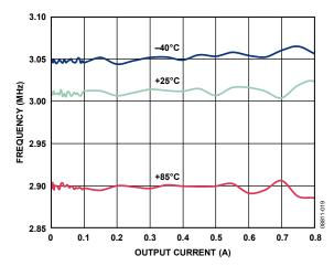
Figure 19. Buck Switching Frequency vs. Output Current, Across Temperature, VOUT1 = 1.8 V, PWM Mode
