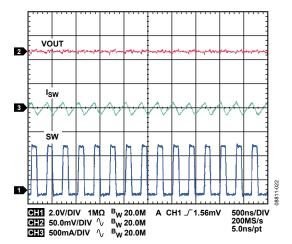
Figure 22. Typical Waveforms, VOUT1 = 1.8 V, IOUT1 = 30 mA, PWM Mode
