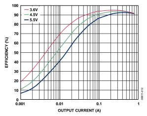
Figure 12. Buck Efficiency vs. Load Current, Across Input Voltage, VOUT1 = 3.3 V, PWM Mode
