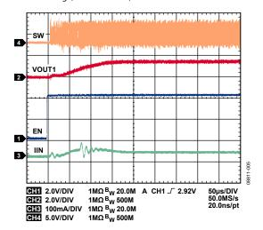
Figure 5. Buck Startup, VOUT1 = 1.8 V,  $I_{OUT1} = 20 \text{ mA}$
