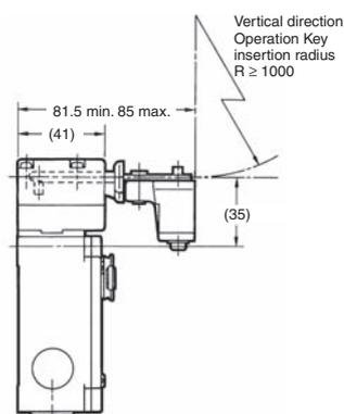
**Note:** 1. Unless otherwise specified, a tolerance of  $\pm 0.4$  mm applies to all dimensions.
