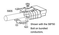
The given wire O.D. information is an estimate. Cable clamps should be evaluated for performance with the actual wire to be used.
