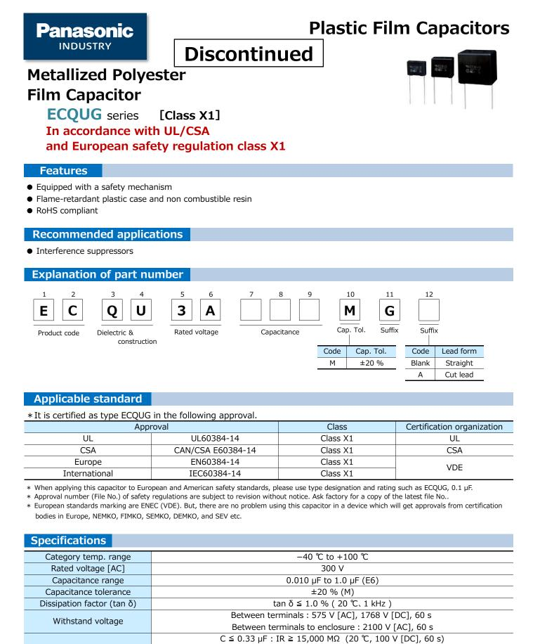
Insulation resistance (IR)  $C > 0.33 \ \mu\text{F} : IR \ge 5,000 \ M\Omega \cdot \mu\text{F} (20 \ C, 100 \ V [DC], 60 \ s)$  $IR \ge 2,000 \ M\Omega (20 \ C, 500 \ V [DC], 60 \ s)$
