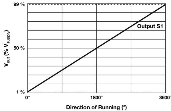
**Redundant Output: with inverted slope**
