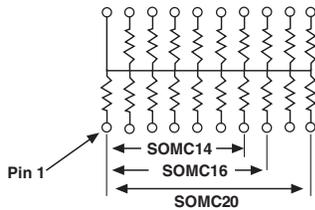
13, 15, or 19 resistors with one pin common
