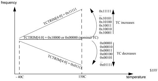
Figure 88. Influence of TCTRIM[4:0] on the Temperature Coefficient
