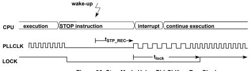
Figure 90. Stop Mode Using PLLCLK as Bus Clock
