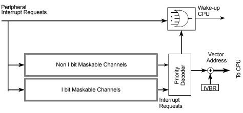
Figure 54. S12SBDMV1 Block Diagram
