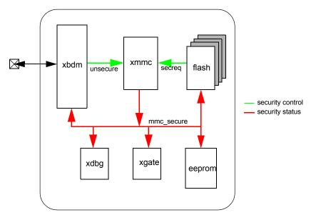
Figure 83. Chip Security Block Diagram
