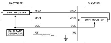
Figure 101. Master/Slave Transfer Block Diagram
