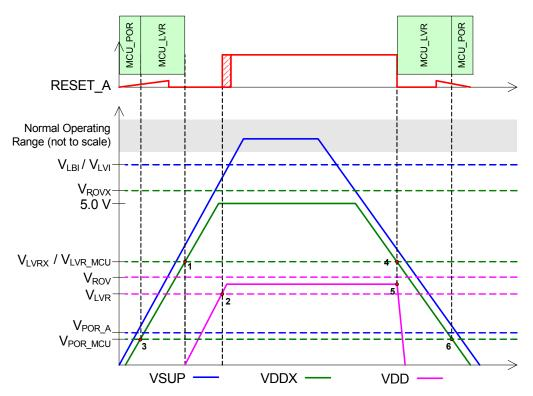
Figure 18. Power Up / Down Sequence
