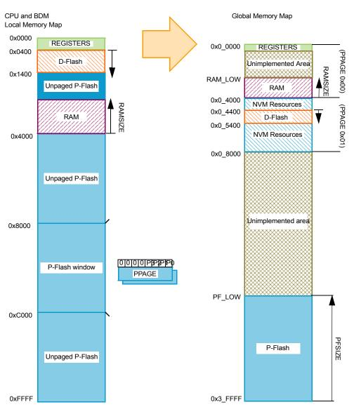
Figure 52. Implemented Global Address Mapping
