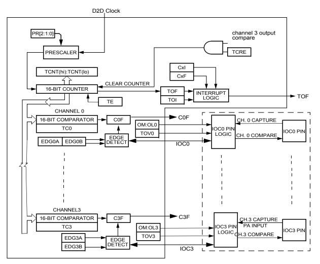
Figure 36. Detailed Timer Block Diagram
