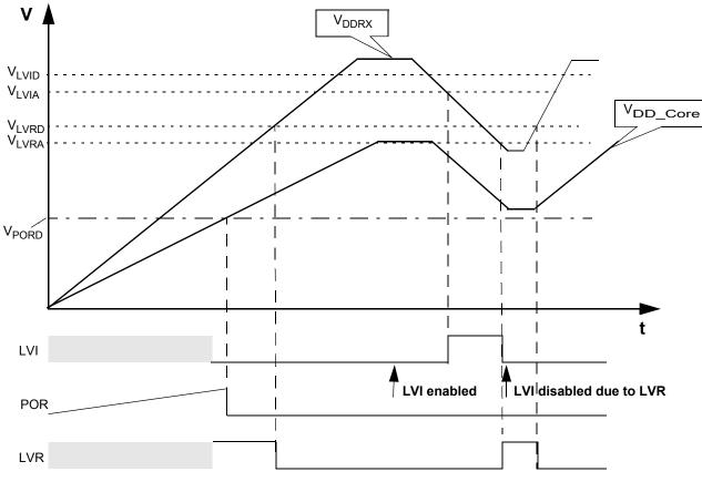
Figure 4. MC9S12I64 - Chip Power-up and Voltage Drops (not scaled)
