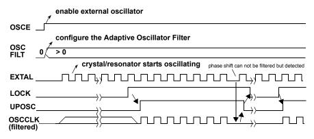
Figure 94. Critical Noise Detected by the Adaptive Oscillator Filter
