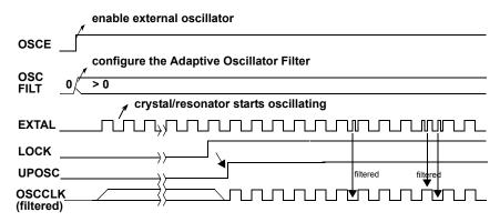
Figure 93. Noise Filtered by the Adaptive Oscillator Filter
