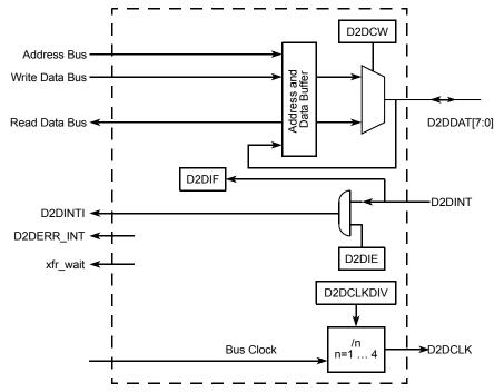
Figure 111. Die-to-Die Initiator (D2DI) Block Diagram
