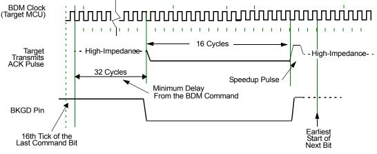
Figure 60. Target Acknowledge Pulse (ACK)
