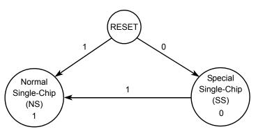
Figure 47. Mode Transition Diagram When MCU is Unsecured
