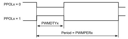
Figure 27. PWM Left Aligned Output Waveform
