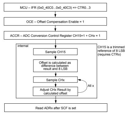
Figure 38. Automatic Offset Compensation
