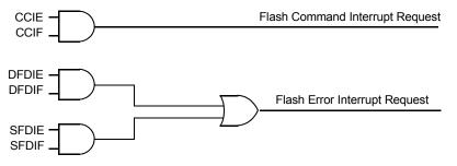
Figure 110. Flash Module Interrupts Implementation
