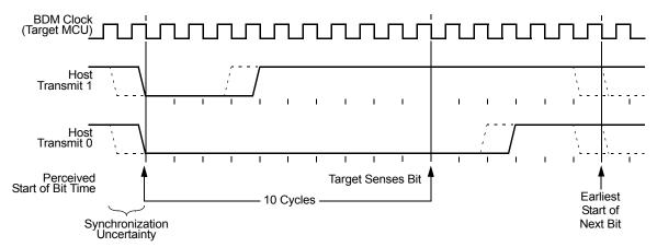
Figure 57. BDM Host-to-Target Serial Bit Timing
