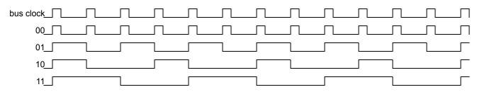
Figure 113. Interface Clock Waveforms for various D2DCLKDIV Encoding
