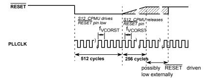
Figure 95. RESET Timing
