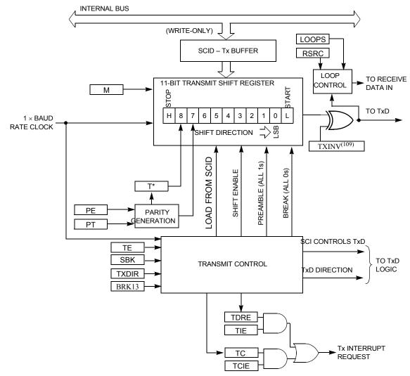
Figure 31. SCI Transmitter Block Diagram
