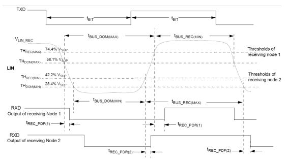
Figure 6. LIN Timing Measurements for Normal Baud Rate
