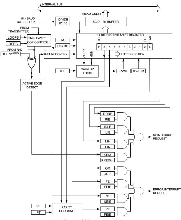
Figure 32. SCI Receiver Block Diagram
