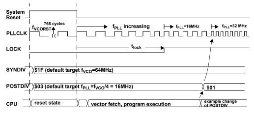
Figure 89. Startup of Clock System After Reset
