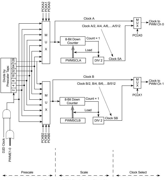
Figure 25. PWM Clock Select Block Diagram
