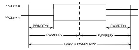
Figure 29. PWM Center Aligned Output Waveform
