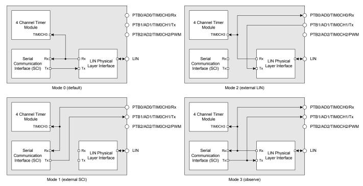
Figure 34. Alternative SCI / LIN Functionality
