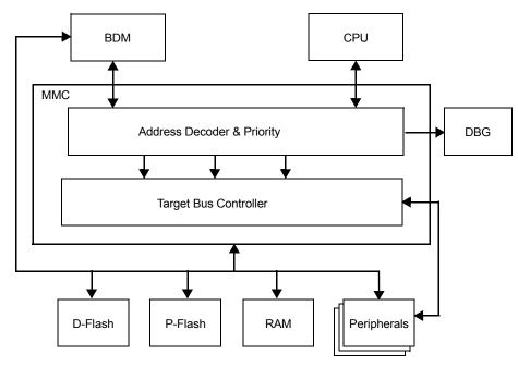
Figure 46. S12PMMC Block Diagram
