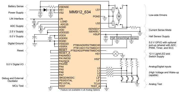
Figure 1. Simplified Application Diagram
