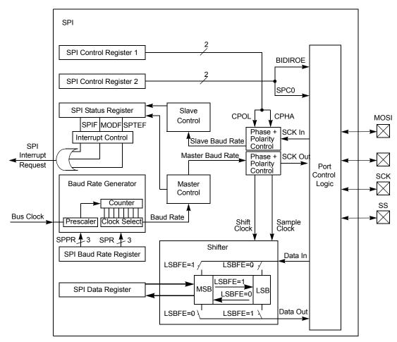
Figure 96. SPI Block Diagram
