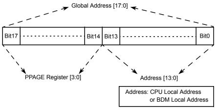
Figure 49. PAGE Address Mapping
