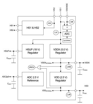
Figure 17. MM912\_634 Power Supply
