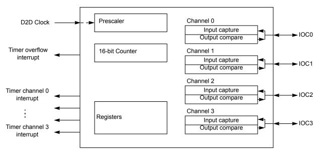
Figure 35. Timer Block Diagram
