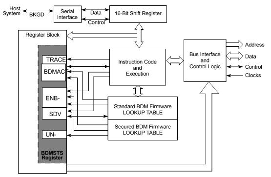
Figure 55. BDM Block Diagram
