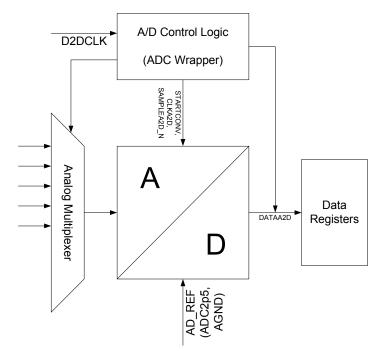
Figure 37. Analog Digital Converter Block Diagram
