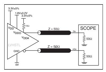
3.3V/1.8V Output Load AC Test Circuit
