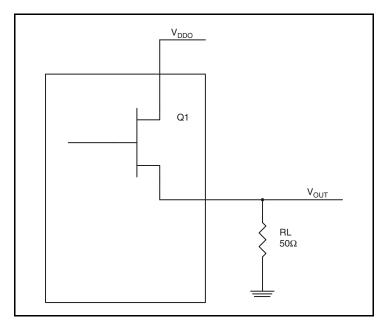
Figure 6. LVHSTL Driver Circuit and Termination
