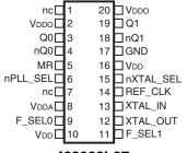
422002I-07 20-Lead TSSOP, EPad 4.4mm x 6.5mm x 0.90mm package body G Package Top View
