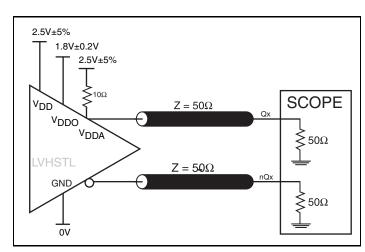
2.5V/1.8V Output Load AC Test Circuit
