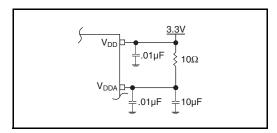
Figure 1. Power Supply Filtering
