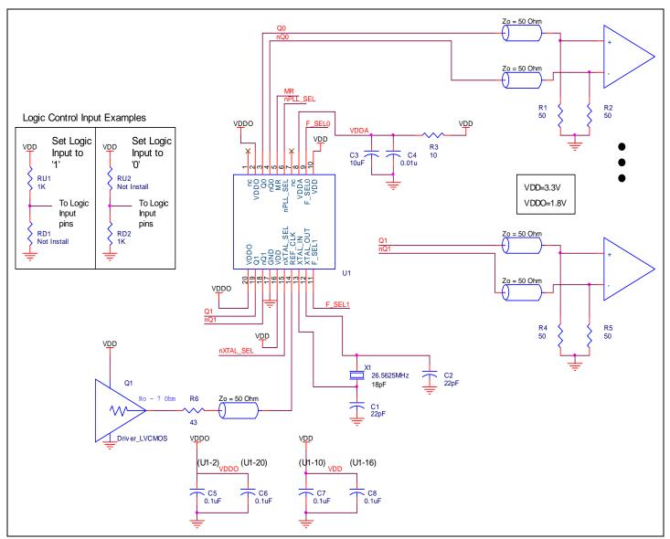
Figure 5. 8422002I-07 LVHSTL Schematic Example
