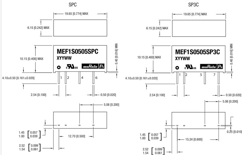
Unless otherwise stated all dimensions in mm (inches)  $\pm 0.05\text{mm}$  (0.002"). Controlling dimension is mm.
