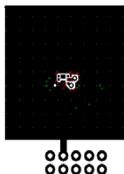
a. 90 °C/W when mounted on a 1 in 2 pad of 2 oz copper.
