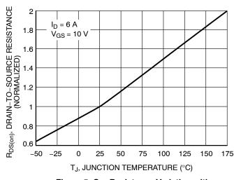
Figure 5. On–Resistance Variation with Temperature
