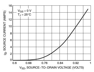
Figure 10. Diode Forward Voltage versus Current
