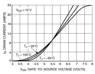
Figure 2. Transfer Characteristics
