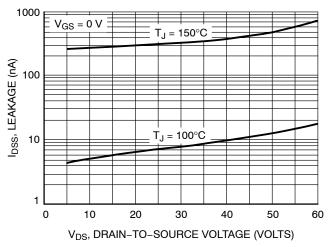
Figure 6. Drain-to-Source Leakage Current versus Voltage
