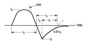
Figure 14. Diode Reverse Recovery Waveform
