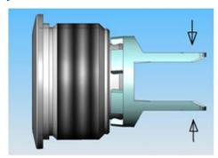
During assembly, the protruding bars of the holder should not be pressed together.
