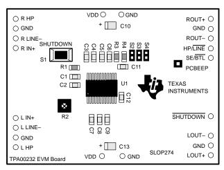
Single in-line header pins extend from the underside of the module circuit board to allow the EVM to be plugged into the TI plug-n-play audio amplifier evaluation platform, or to be wired directly into existing circuits and equipment when used stand-alone.
