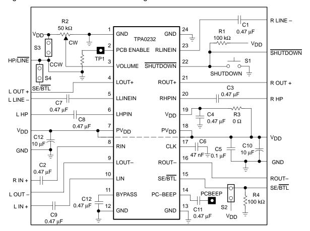
Figure 3-3. TPA0232 EVM Schematic Diagram
