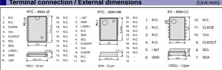
The metal case inside of the molding compound may be exposed on the top or bottom of this product
