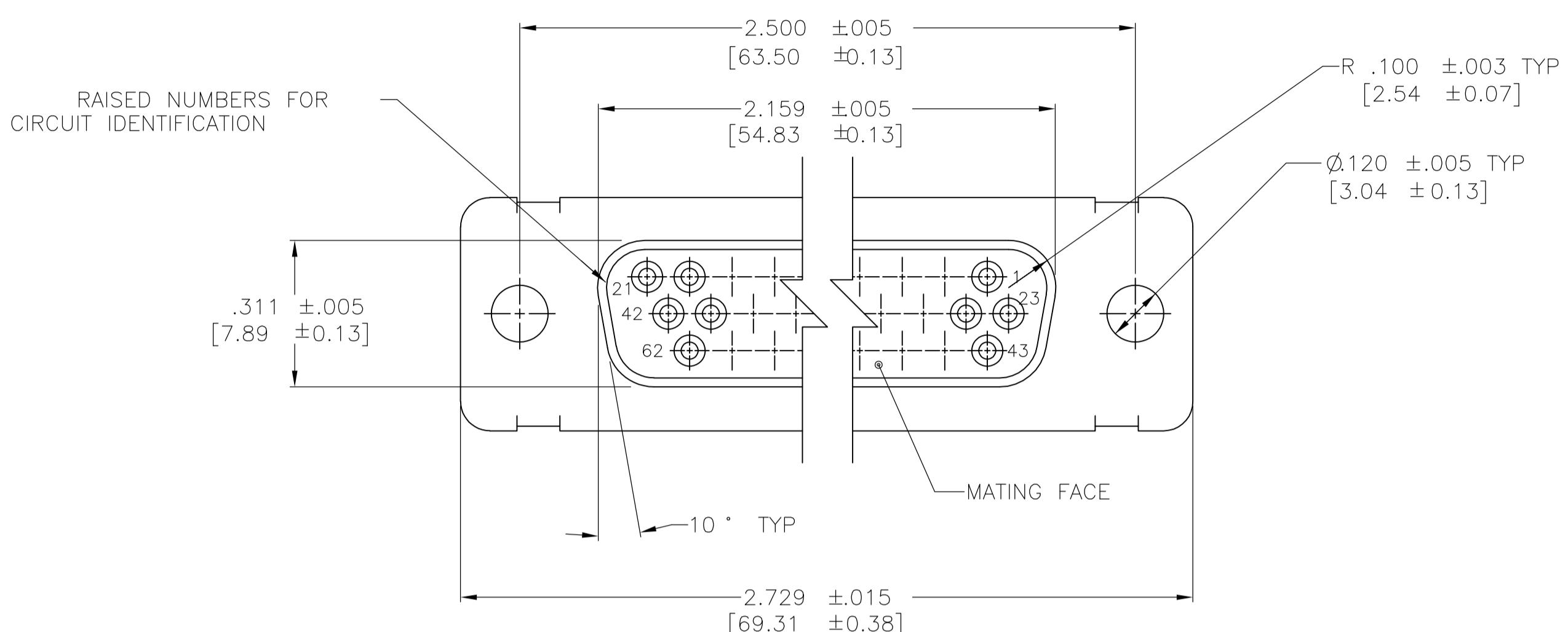
1. THIS RECEPTACLE WILL MATE WITH ANY SIZE 4, 62 POSN. PLUG IN AMPLIMITE SERIES.
