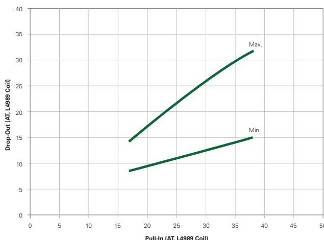
Note: The chart represents the range of Drop-Out, minimum to maximum for a given Pull-In value.
