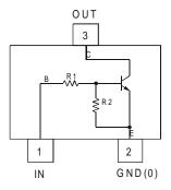
Schematic and Pin Diagram
